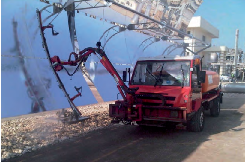
Figure 3.1.2.2: Cleaning a solar trough power plant, Kuraymat, Egypt. | Source: Gerhard Hofmann, Agentur Zukunft.
