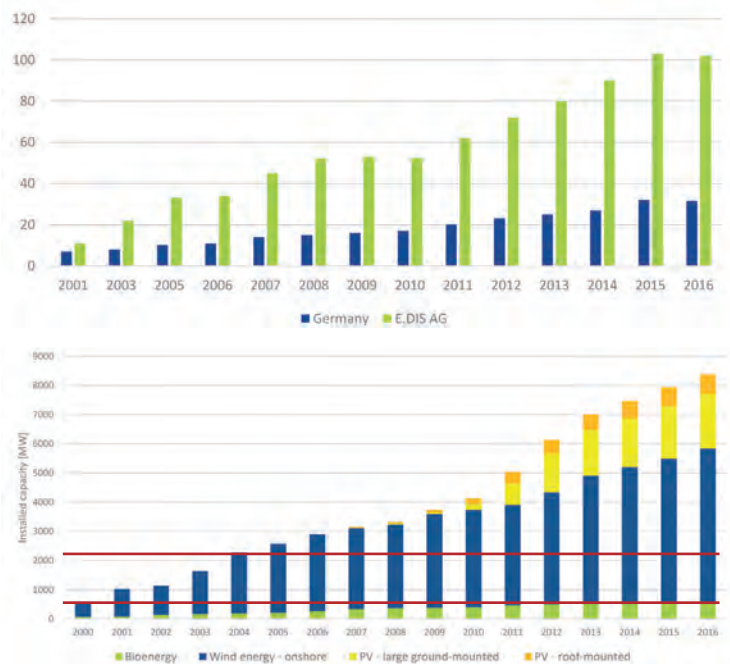
Figure 3.2.1.1.1: Bar chart A: Renewable energy generated in E.DIS grid network region (red bars) is more than 100% of what the E.DIS grid extracts and distributes to end-users. The average for the whole of Germany is 33% (dark blue bars). Bar chart B: Installed renewable energy capacity in the E.DIS grid network region is greater than the peak load on the E.DIS by a factor of 4, and the baseload by a factor of 17. | Source: Prof. Dr. H. Schwarz, b-tu.de: e.dis. | Graphic: RENAC.
